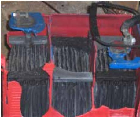
Fig. 56: Blown batteries
