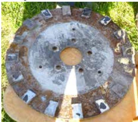
Fig. 65: Rusted rotor
