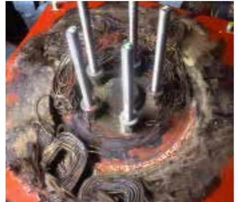
Fig. 61: Burnt stator
