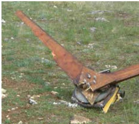
Fig. 63: Loss of balancing weight
