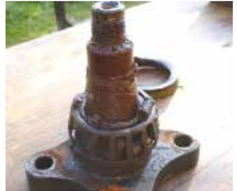
Fig. 58: Broken bearing
