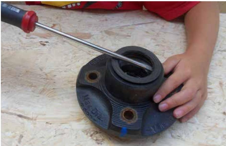
Fig. 37: Remove the seal
